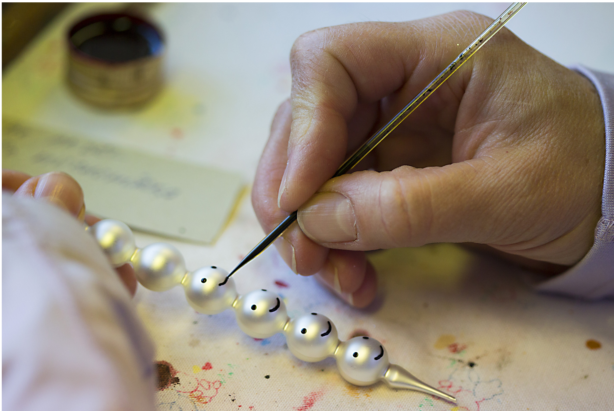
Photo no. 6 Hand made Production of Christmas Tree Decorations from blown glass Beads; painting of semi-finished products
