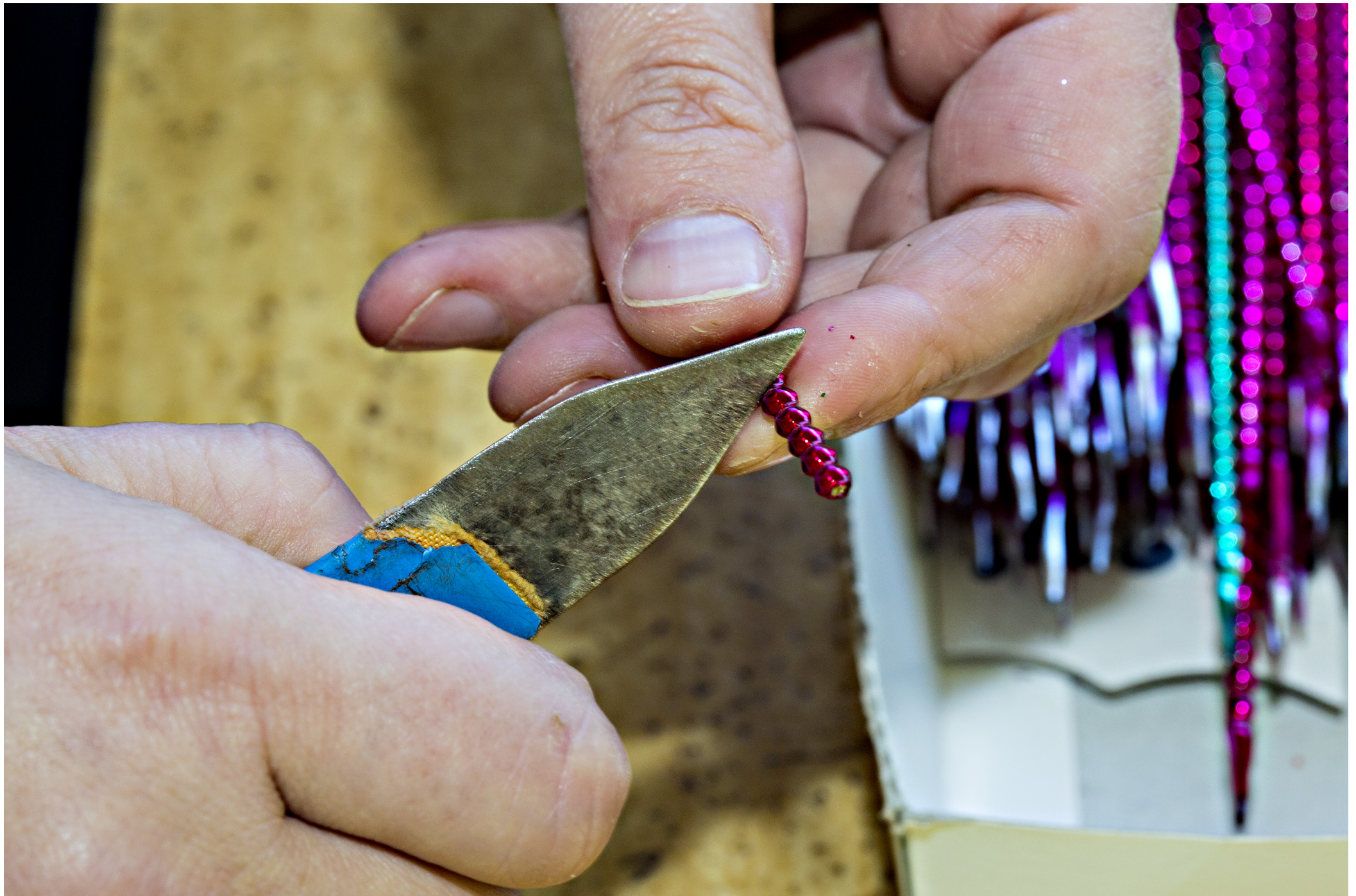
Photo no. 7 Hand made Production of Christmas Tree Decorations from blown glass Beads; cutting of preforms
