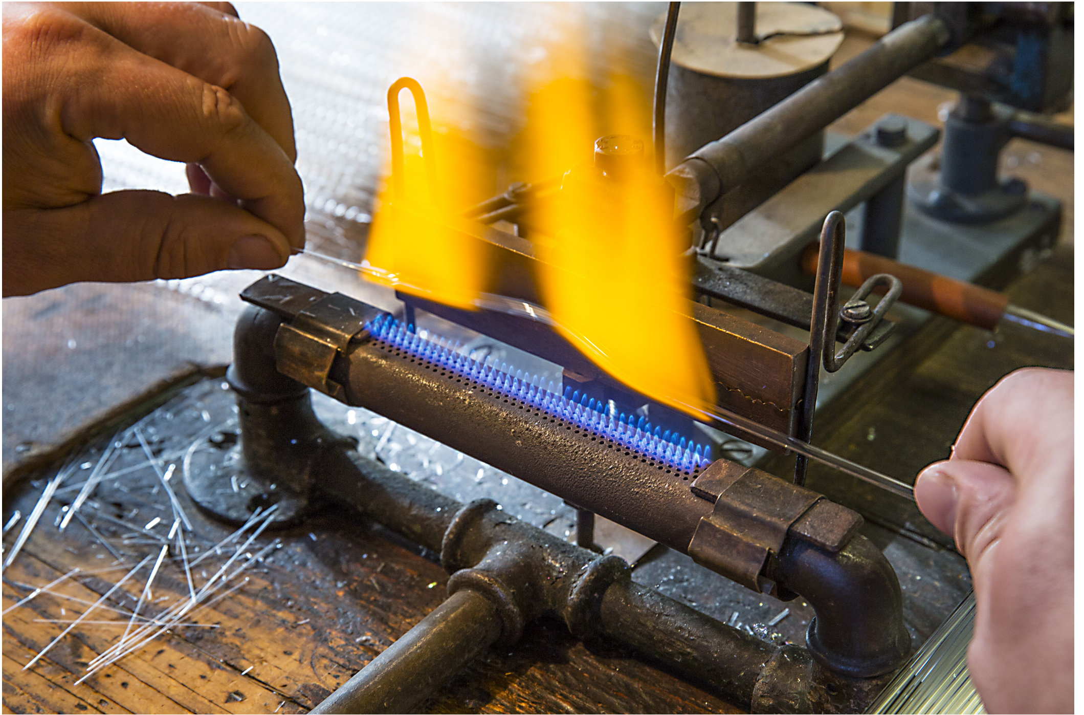
Photo no. 3 Hand made Production of Christmas Tree Decorations from blown glass Beads; heating of the hollow glass tube over a burner
